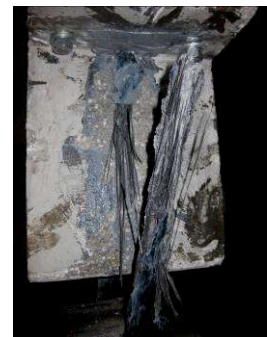
Fig. 10d. Failure mode of specimen CFRP Rope SWFX No 2
